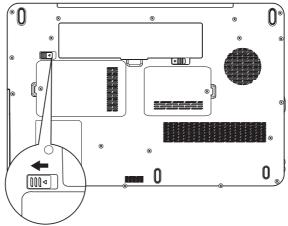
Figure 6-1 Releasing the battery pack (1)
